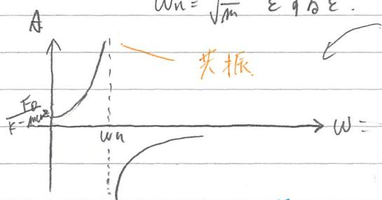
$$\Downarrow \quad x = \frac{|F_0/m|}{(\omega_n^2 - \omega^2)} \sin(\omega t + \phi), \quad \phi = \begin{cases} 0 & (\omega < \omega_n) \\ \pi & (\omega > \omega_n) \end{cases}$$
