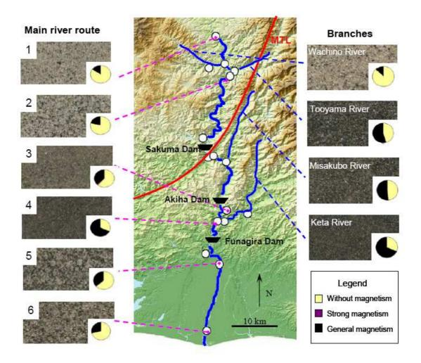
Fig. 6 Surface sand samples on the Tenryu watershed
