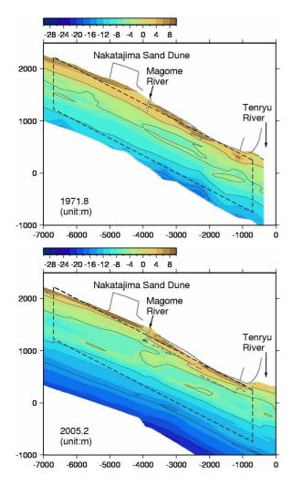
Fig. 2 Nearshore bathymetries of Hamamatsu Coast (1971 and 2005)
