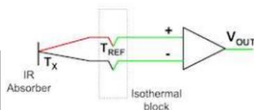
$$V_{OUT} = S \cdot (T_X - T_{REF})$$
